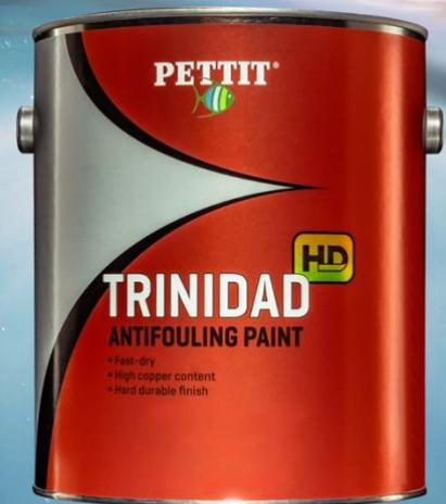
**APPLICATION SYSTEMS:** Trinidad HD is easily applied by brush, roller or spray. When rolling, use only a high-quality short nap (maximum 1/4" nap) roller cover. Over-application of this product will virtually assure inadequate coating performance. Mix paint thoroughly to ensure ingredients are evenly dispersed throughout the can. All surfaces must be clean, dry and properly prepared prior to painting.
